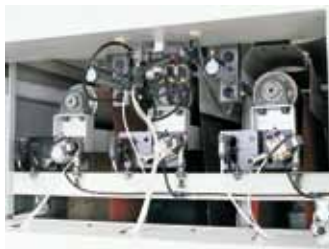
Schleifbandreinigung blower device to clear sanding belts
