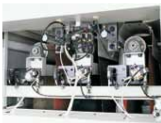
Schleifbandreinigung blower device to clear sanding belts
