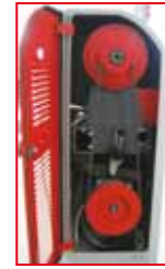
stabiler Riemenantrieb solid and smooth belt run
