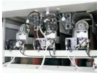
Schleifbandreinigung blower device to clear sanding belts
